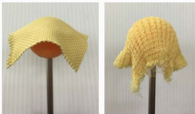
Fig. 7. Qualitative assessment of the auxetic properties: Woven vs. Auxetic Kevlar
