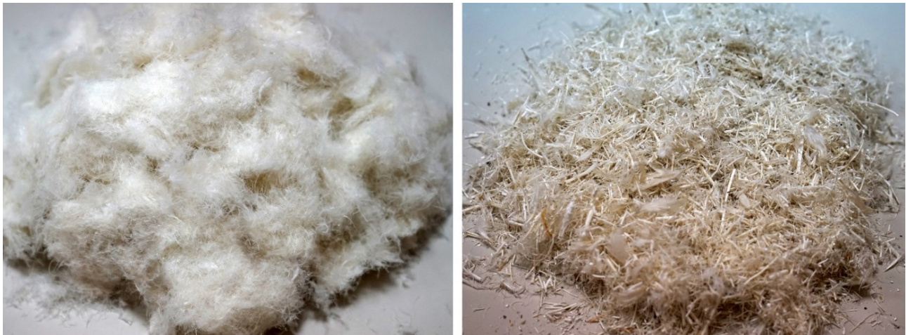
Fig. 1. Fibers which were obtained from chicken feathers (left) and separated rachis (right)
