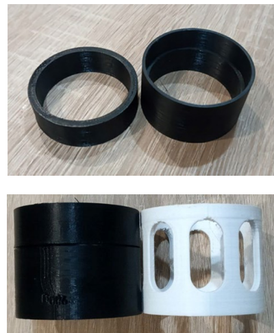
Figure 1. Examples of nozzles for standard coils on the left and custom nozzle on the right
